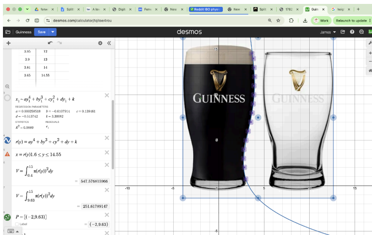
Figure 2. Tracing the cavity edge in Desmos, with the photograph calibrated to centimetres.
